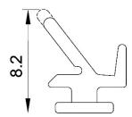
This seal is the standard frame seal for Air Flo & Carinya Hinge doors as it has replaced the QLON-48650FR seal which was previously required for bushfire requirements. This results in using one seal for all site conditions. The description has changed from AFD002 to AFD002FR to reflect this material change keeping the same item number. Stock will transition as it runs out as some branches are already supplying the improved product.
